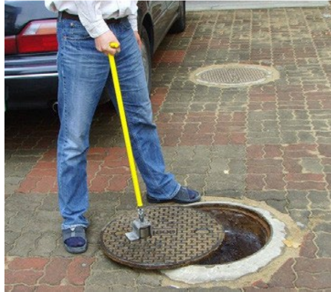
HLF-R5040-L Weight: 3.3kg Max Load: 50kg
