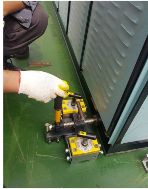
Model: Stopper-4000-Bite (2 x Stopper-2000-Bite) Max Force: 4Ton Weight: 49Kg Dimension: 310W x 678L x 856H
