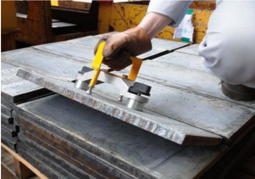
HLF-R5040-S Weight: 1.8kg Max Load: 50kg
