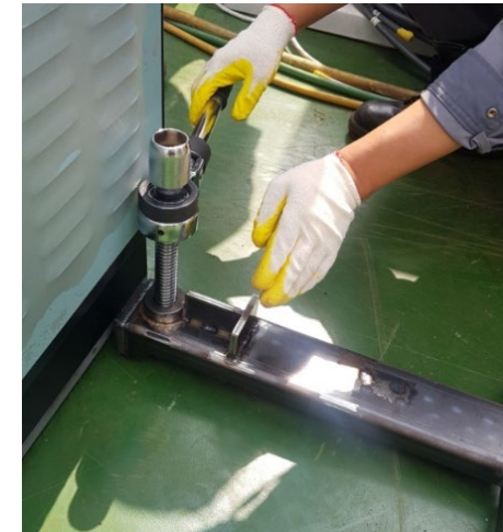
Model: Ratchet-Jacky-1000 For Corner Lifting
