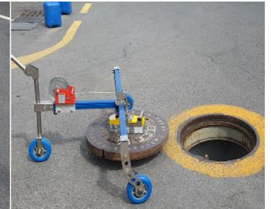
Move the manhole cover
